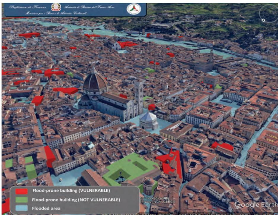
22. Georeferenced system to identify vulnerable areas in support of the Florence flood alert system.
