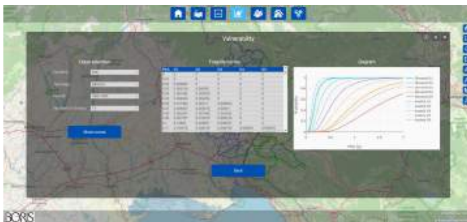
Figure 3.16: Visualization of an example of the seismic fragility curves for the Pilot 2 area on the BORIS platform.
