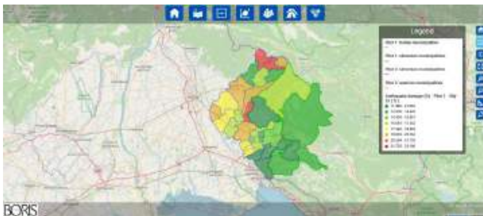
Figure 2.14: Percentage of buildings in D1 for seismic risk in Pilot 1: a) in 1 year; b) in 50 years.
