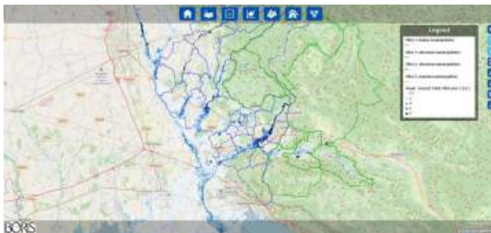
Figure 2.19: Flood hazard map for Pilot 1 considering an event with a return period of 500 years.
