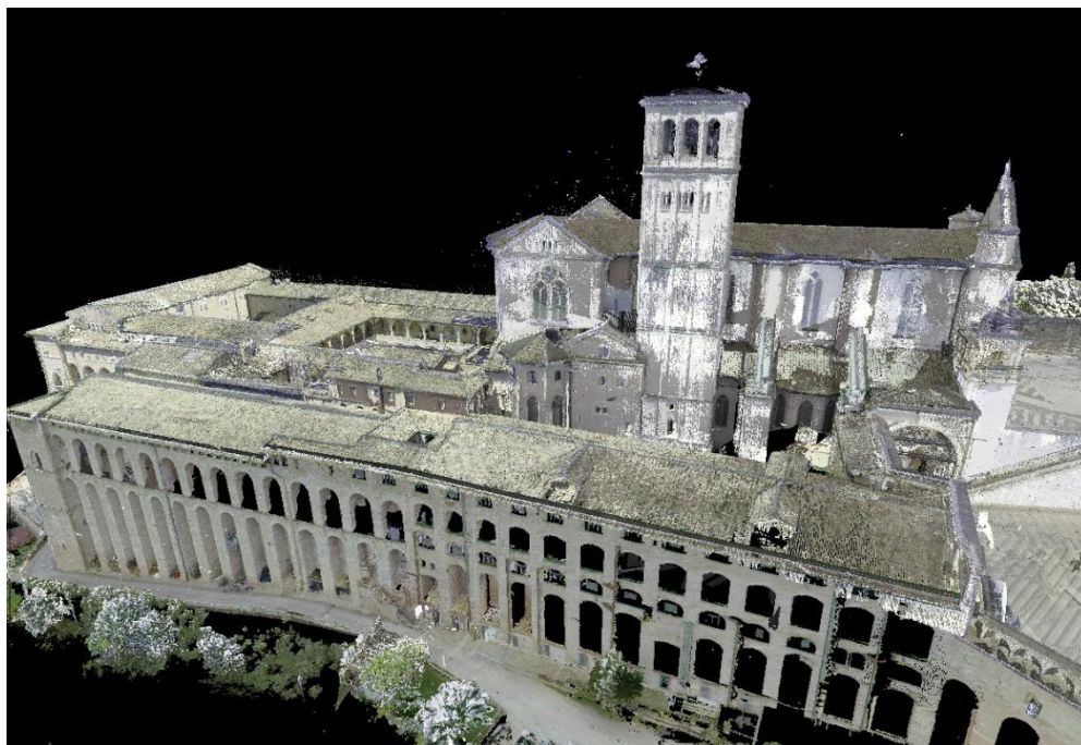
Fig. 9 Sacro Convento of Assisi: 3D point cloud perspective © Vigili del Fuoco
