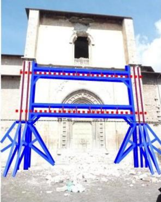
Fig. 3 Church of San Domenico (L'Aquila): design of provisional works © Vigili del Fuoco
