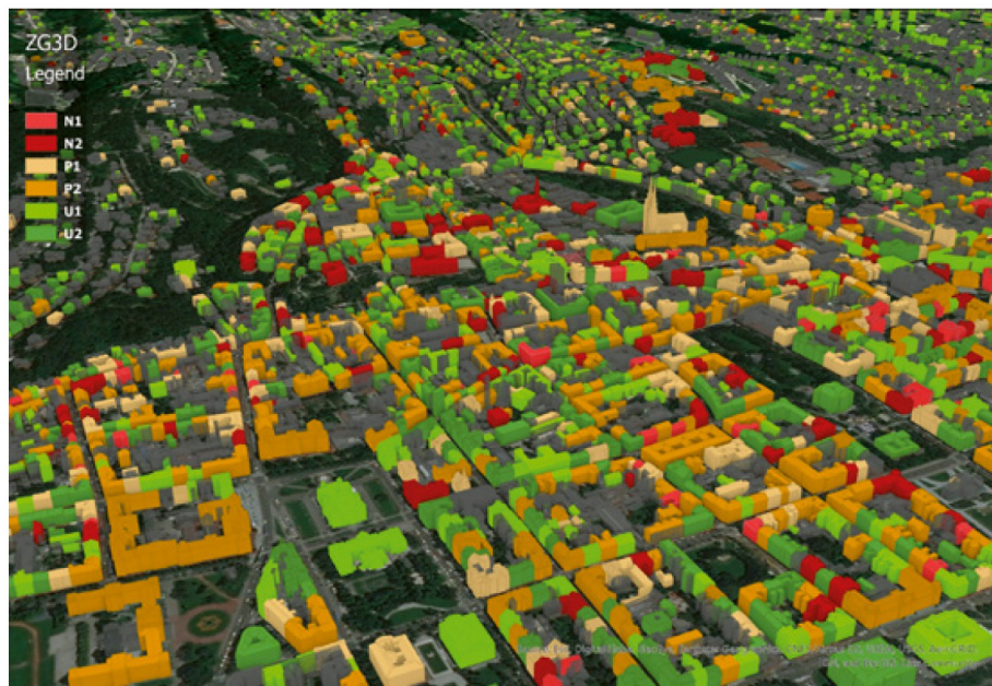
Figure 1.12 3D view of the Lower and Upper Towns of the City of Zagreb based on the usability classifications (Croatia Earthquake RDNA, 2020)
