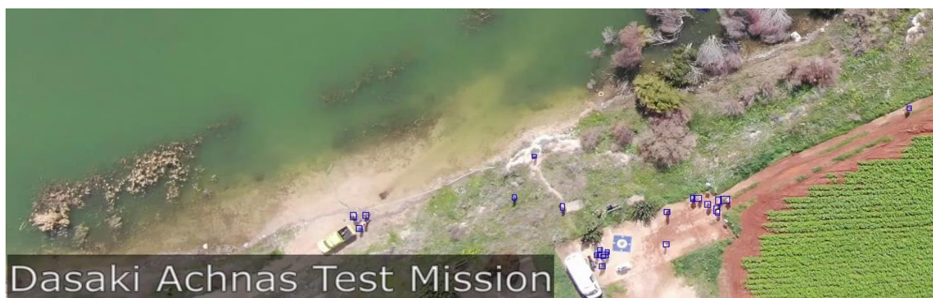
Figure 14: A screenshot from a video captured during a field exercise where all persons are detected (marked with blue boxes)
