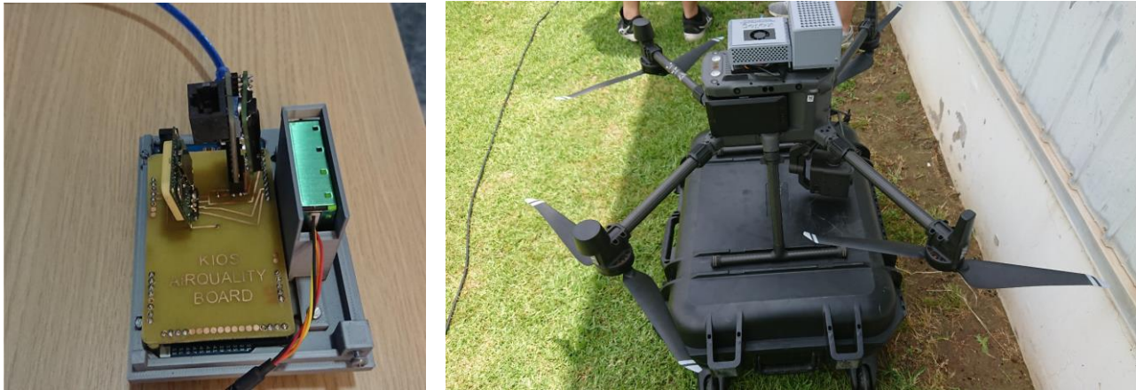
Figure 10: The developed hardware board equipped with air quality sensors (left) and the board attached to the UAV (right)
