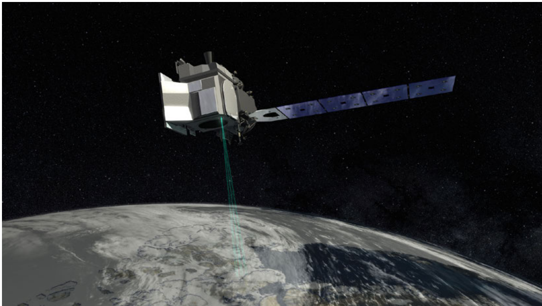
Figure 7.1 ICESat-2 satellite - a laser altimetry satellite measuring polar ice, sea level and forest canopy
