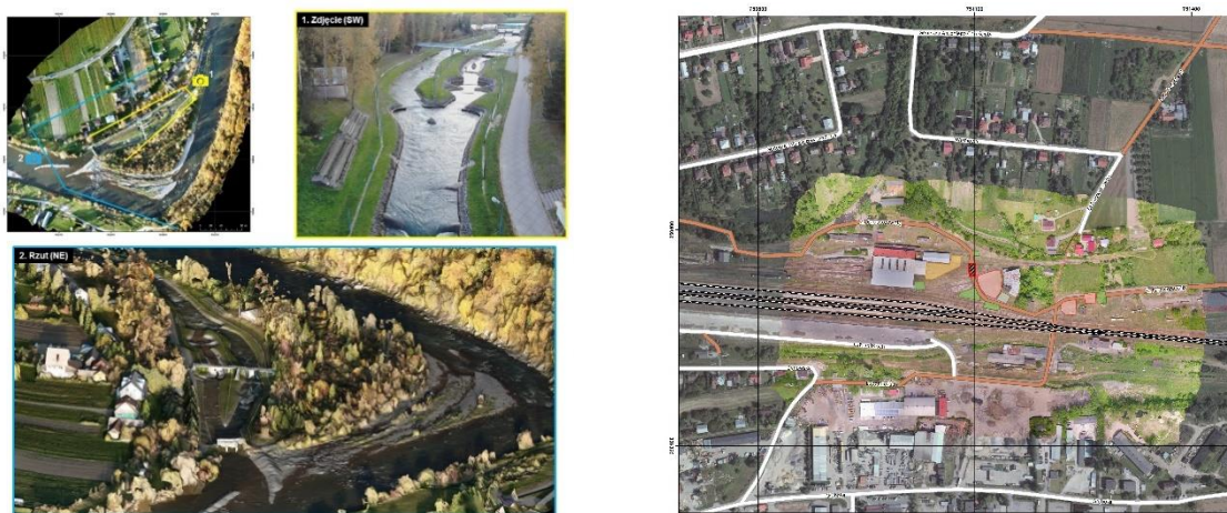
Figure 2.2. Information materials derived from drones flying automatically over the site. From left: a photo and 3d model of a mountain river bend; a detailed ad-hoc mosaic overlaid on an older aerial photo and with a visible diagram of the road infrastructure. Such products can today be processed on the fly or within minutes via cloud-based processing unit. Collected and processed by CIK in 2018.
