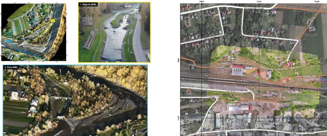
Figure 2.2. Information materials derived from drones flying automatically over the site. From left: a photo and 3d model of a mountain river bend; a detailed ad-hoc mosaic overlaid on an older aerial photo and with a visible diagram of the road infrastructure. Such products can today be processed on the fly or within minutes via cloud-based processing unit. Collected and processed by CIK in 2018.
