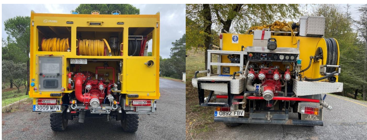
Figure 19: Pump assembly at a new generation (left) and an old generation (right) heavy firefighting truck
