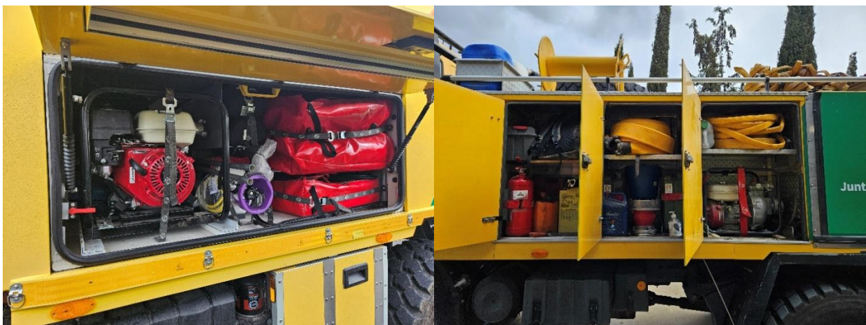
Figure 21: Equipment compartments at a new generation (left) and an old generation (right) heavy firefighting truck
