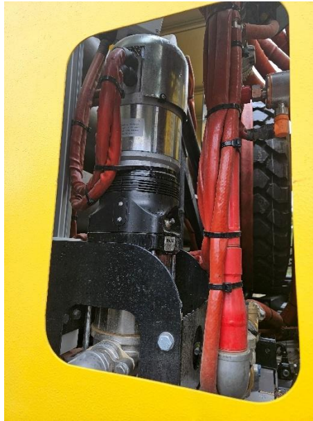
Figure 20: Electrical pump for the trucks self defense system, located in the back of the cabin
