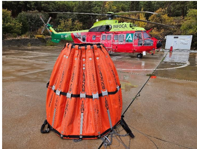
Figure 15: INFOCA Helicopter with 3000 l Bambi Bucket
