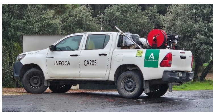
Figure 22: 4x4 Quick attack unit with 400 l of water capacity used to tackle spot fires
