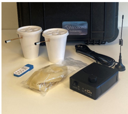
Figure 5. Radiosondes launching equipment. Reference: Windsound.
