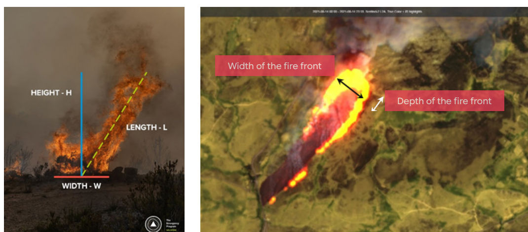
Figure 7. Left: Definition of flame length. Reference: The Emergency Program (TEP). Right: Definition of the width and depth of the fire front on a Sentinel 2 image from the Avila wildfire (August 2021, Spain). Reference: SentinelHub.
