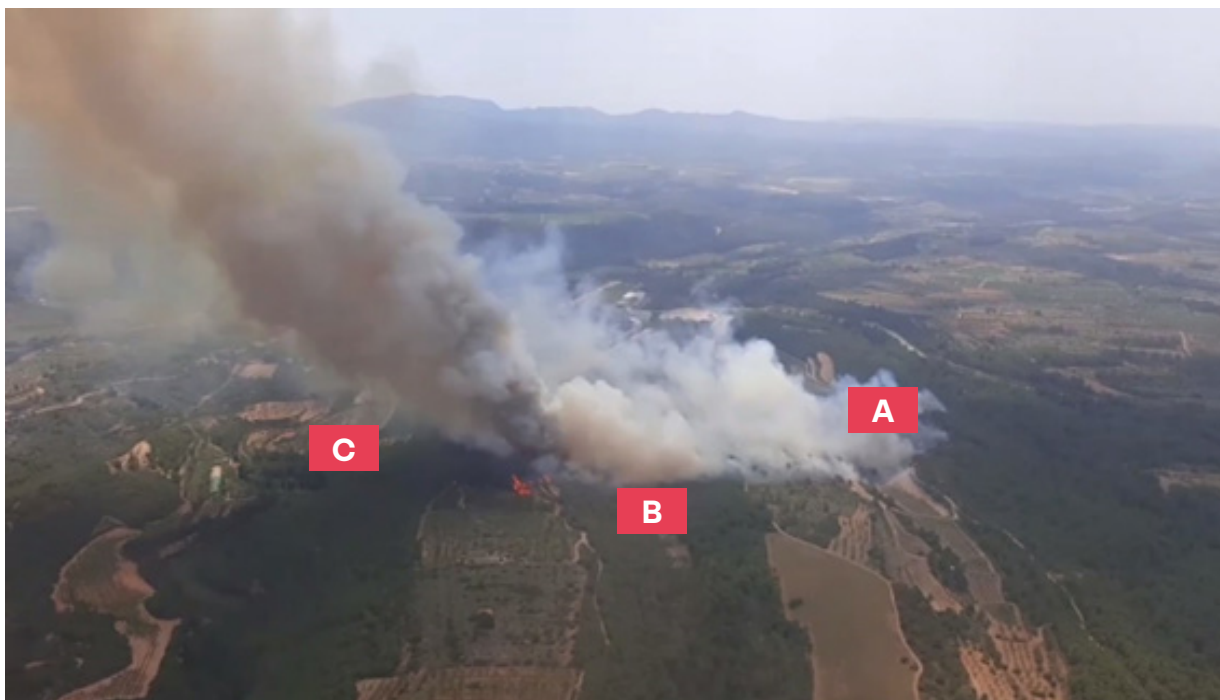
Figure 2. The launching position of a radiosonde in a wildfire. A: from the back of the fire, B: from the flanks, C: from the head of the fire. Reference: CFRS.
