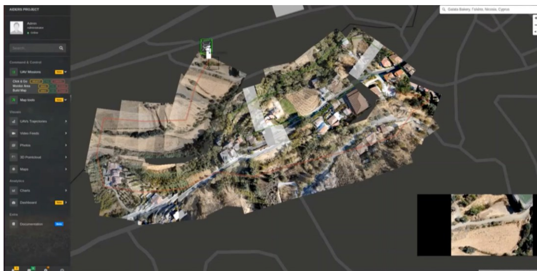
Figure 8: Orthomosaic map generation through UAS images [19].
