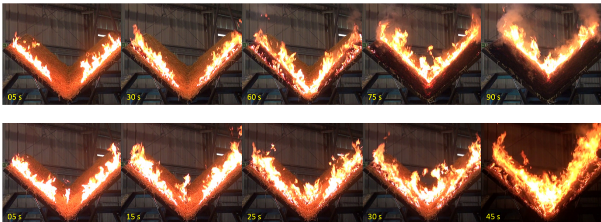
Figure 24. Sequence of frames from two laboratory tests in a canyon (water line slope: 15°; versant slopes: 30°) with the same fuel conditions: top row - two fire fronts; bottom row - two fire fronts and a fire ignition.
