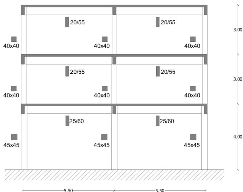
Figure 66. Geometry of a simplified concrete frame
