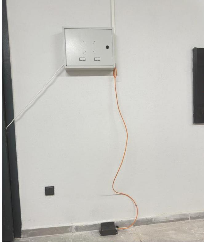
Figure 29. Çamkiran Ortaokulu Bayraklı 3<sup>rd</sup> Floor Accelerometer Location (Instrumentation).
