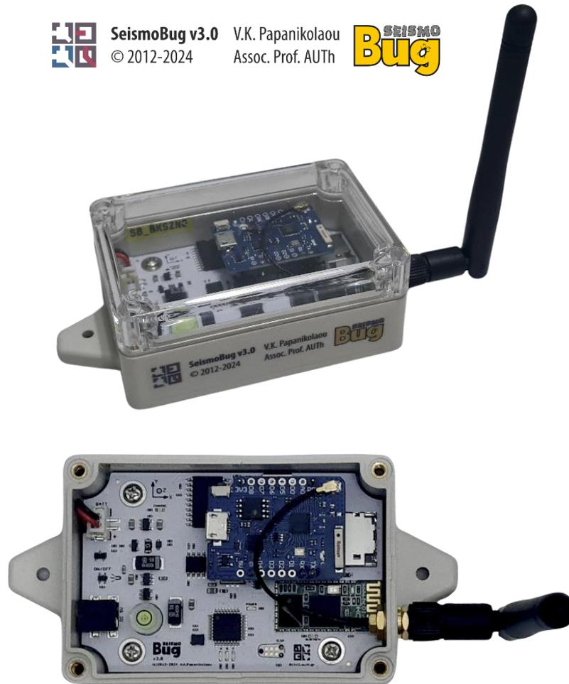
Figure 1. The low-cost accelerometer SeismoBug v3.0.
