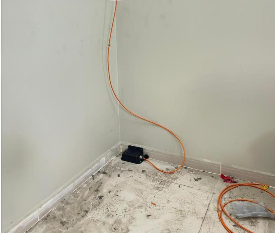
**Figure 31.** Bornova Anadolu Lisesi G-Blok 2<sup>nd</sup> Floor Accelerometer Location (Instrumentation).
