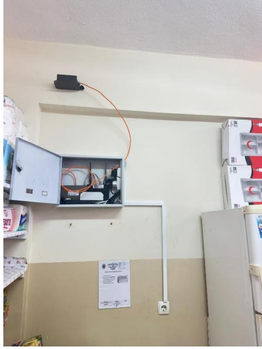
Figure 27. Ali Osman Konakçı Mesleki ve Teknik Anadolu Lisesi 3<sup>rd</sup> Floor Accelerometer Location (Instrumentation).
