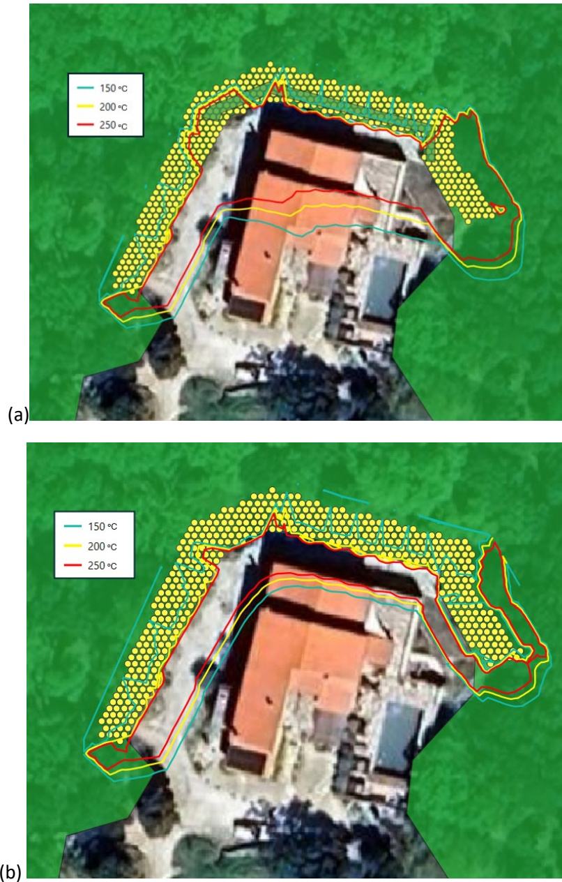
Figure 4-2 : incident temperature isolines issued by SWIFFT model: (a) with flammable ornamental hedge, (b) with non-easily flammable ornamental hedge
