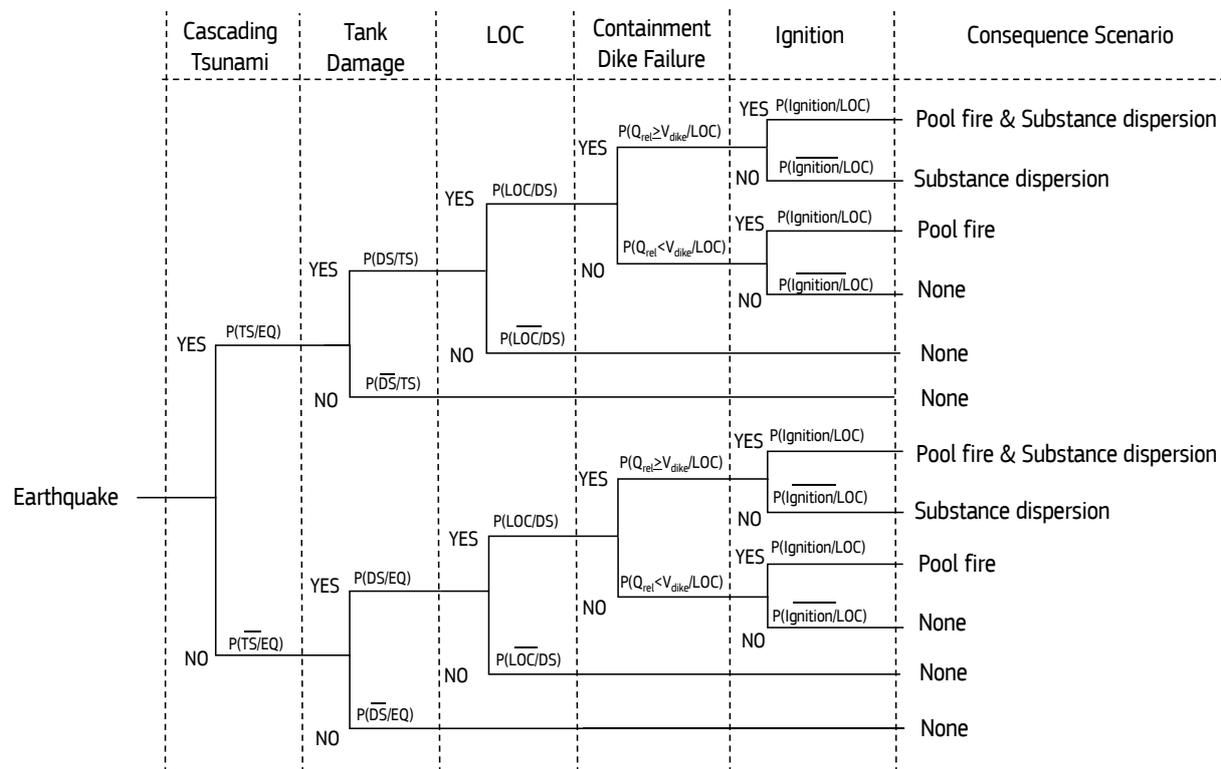
By integrating the above considerations into the event tree of Figure 14, this is expanded to the one shown in Figure 22, which comprises the following events:
