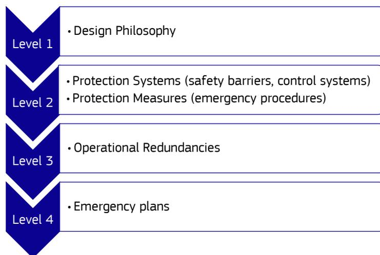
At the first level lies the **design philosophy** for the construction of new hazardous sites or the retrofit of existing ones. The aim of the design philosophy is to provide robust structural systems that withstand external actions from natural and man-made hazards. In this respect, the developed design
