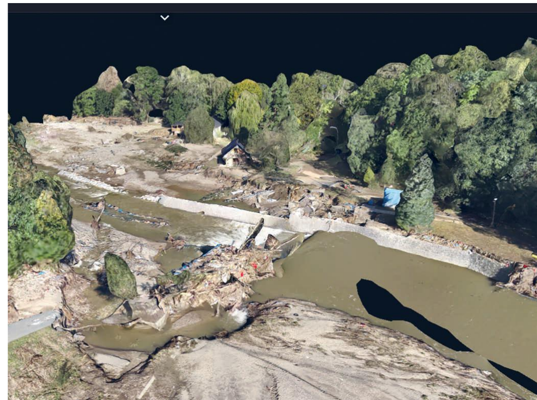
Water sill on the Gluchotaska Biala River. Measurable 3D model created after the passage of a destructive flood wave. Made by drone due to the very difficult access to the site by land. At the same time, the model allows a numerical and quantitative assessment of the restoration of access roads to the site. In addition, it provides information on the amount of dry material needed to restore the river to its natural channel.
