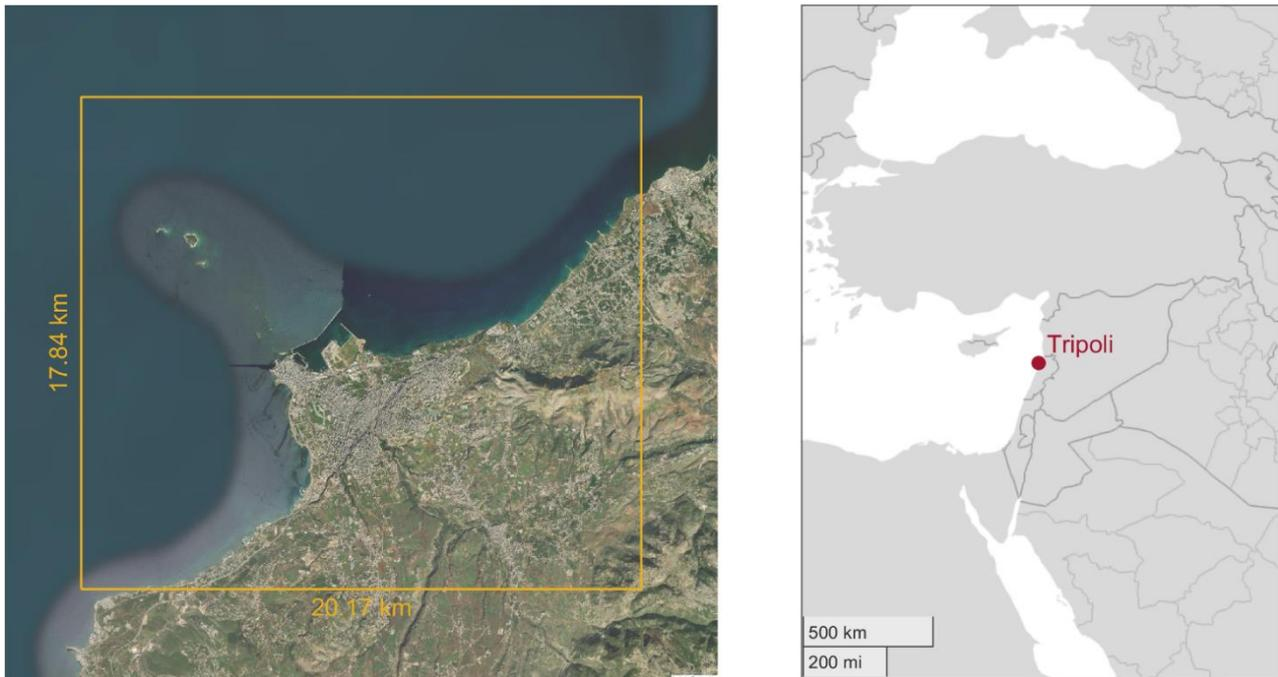
Figure 3. Plan view of the Tripoli harbor's computational domain
