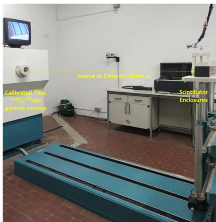
Figure 11. Setup of the measurements performed to investigate the energy dependence of the intrinsic photopeak efficiency of the detectors.
