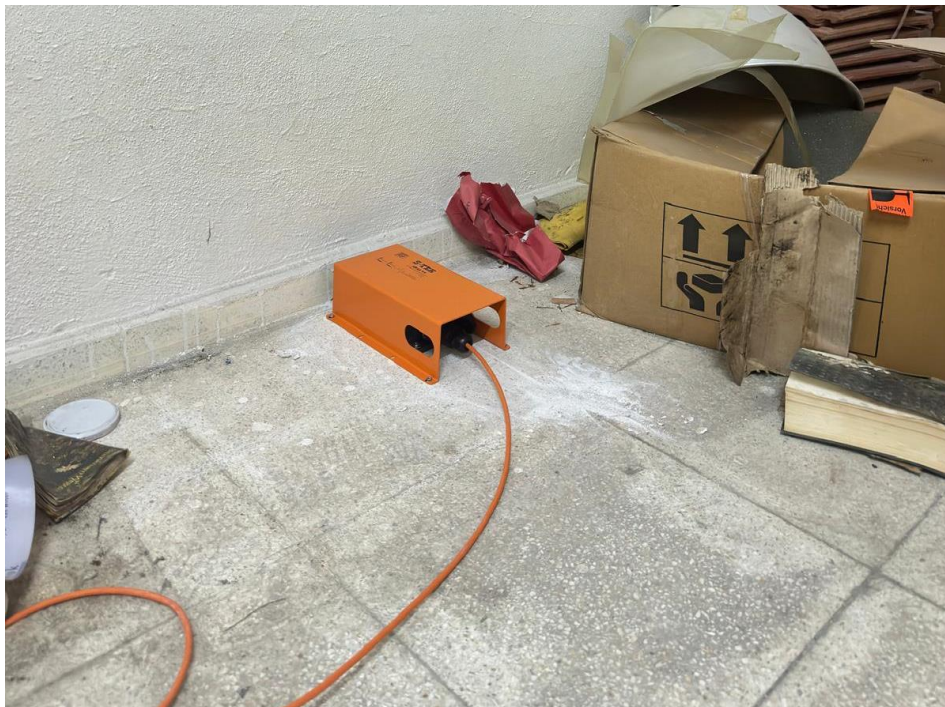
Figure 32. Bornova Anadolu Lisesi G-Blok Basement Floor Accelerometer Location (Instrumentation).
