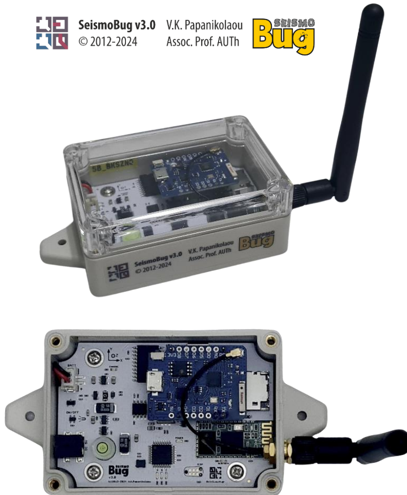
Figure 1. The low-cost accelerograph SeismoBug v3.0.
