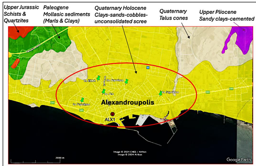
Figure 12. Geologic map of the broader area of the city of Alexandroupolis together with the 5 selected school units (1:50.000 scale, IGME maps, https://www.eagme.gr/site/services ). The ITSAK permanent accelerometer station is also shown as ALX1.
