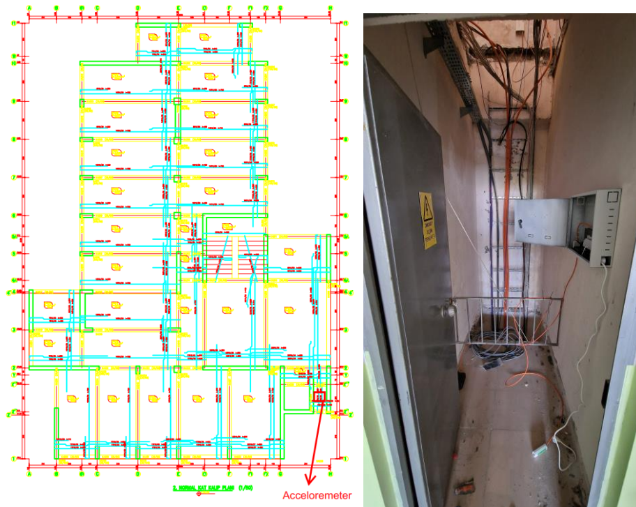
Figure 40. Gelibolu 100. Yıl Barış Ortaokulu 3 rd Floor Accelerometer Location (floor plan (left), instrumentation (right)).
