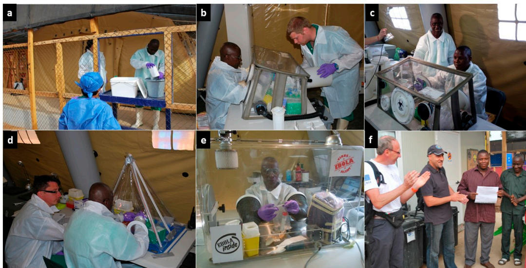
Figure 4. Biosafety training and qPCR procedures. A double fence surrounded the laboratory, the first to control entry to the site and perform biosafety measures (temperature monitoring, hand and shoe decontamination), the second to restrict access to the laboratory staff. (a) Samples were received through a window in the internal fence. The training focused on handling Ebola samples inside a negative-pressure glovebox, (b) first under supervision and then (c) autonomously, (d) to prepare a 96-multiwell plate for the qPCR inside a disposable glovebox, and (e) to perform biochemical tests. (f) Certificates of attendance were issued at the end of the JiTT program.
