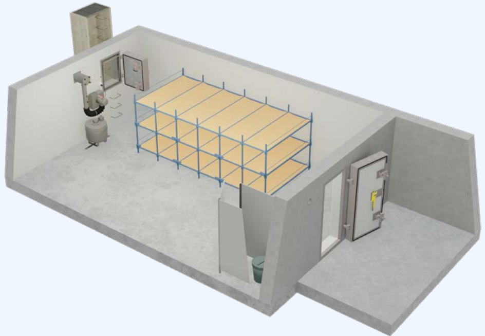
Image 9 The required equipment consists of bunk beds and dry toilets. They must be brought into the shelter and set up according to the instructions.
