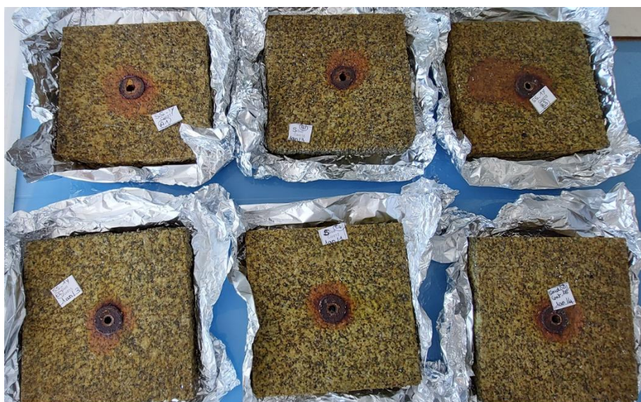
Figure 58 Pictures of the control tiles from the South face of the quay, after 11 months of exposure, at the laboratory before extraction
