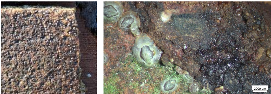
Figure 60 (left) Tile covered with HFO, at T4 (6 months), the little white dots are barnacles, (right) picture taken with the binocular loupe in Cedre's laboratory
