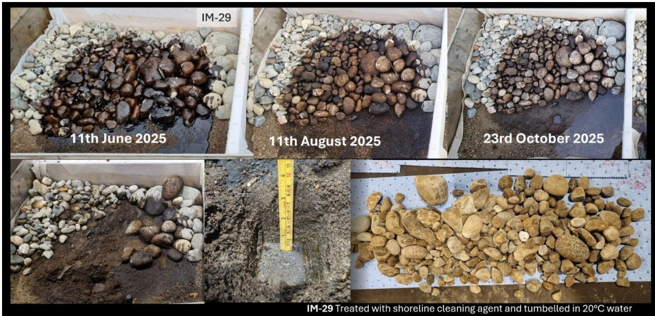
Figure 90: Weathering of IM-29.
