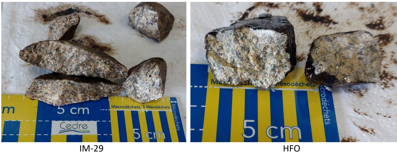
Figure 78 Pictures of pebbles collected in the tanks at the end of the trials, showing the oil penetration for the three LSFOs
