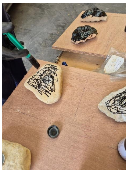
Figure 15 Addition of oil on the rocks used for the trials in Malta
