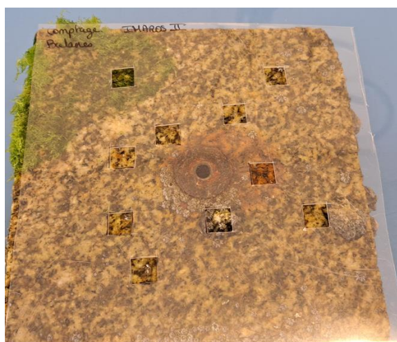
Figure 21 Frame used to evaluate the number of barnacles
