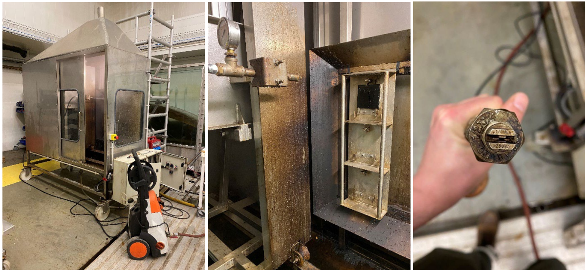
Figure 1 Pictures showing the Flushing Robot, the steel rack holding the tiles and the nozzle.
