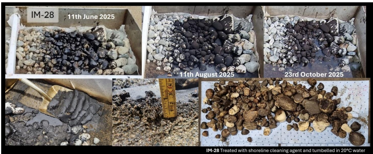
Figure 88: Weathering of IM-28.
