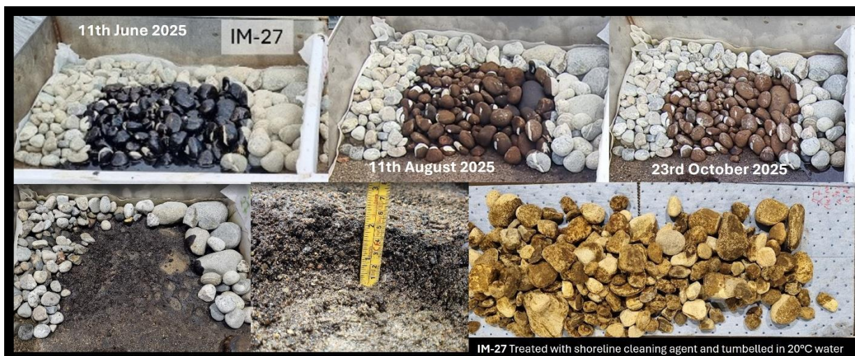
Figure 86: Weathering of IM-27.
