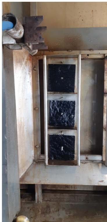
Figure 5 Installation of tiles in the washing robot
