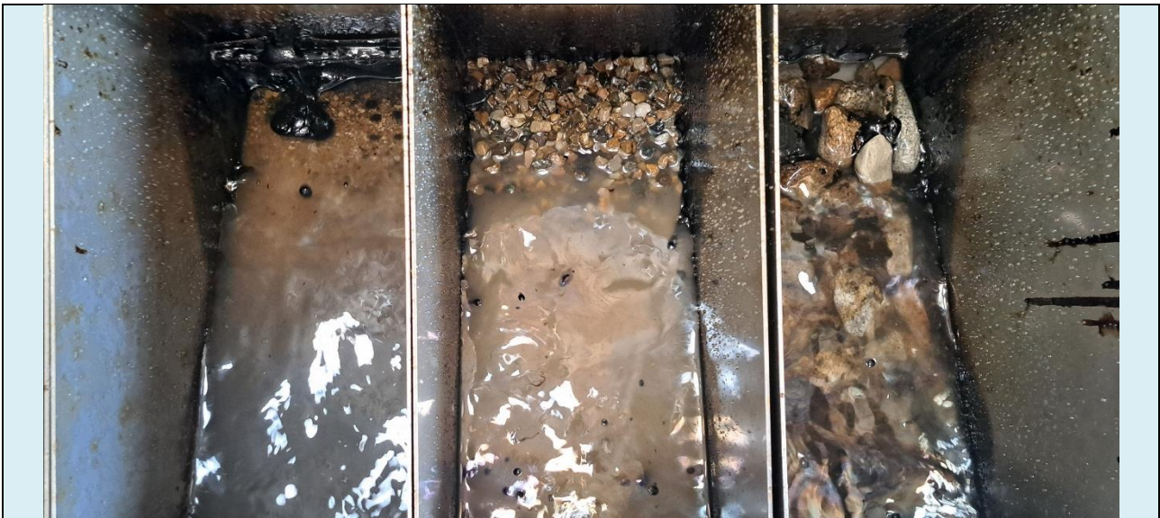
Little remobilisation of the oil that mainly stick to the walls. Oil trapped in the sediment does not easily resurface and stays stuck on the manual tools when mixing the sediment.
