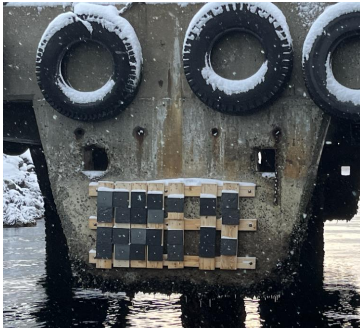
Figure 64 Picture of the tiles after 15 days of exposure
