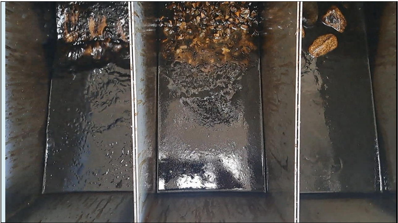
Easy remobilisation of the oil present on the top of the sediment leaving the surface sediment almost cleaned. Trapped oil needs manual agitation of the sediment to resurface.
