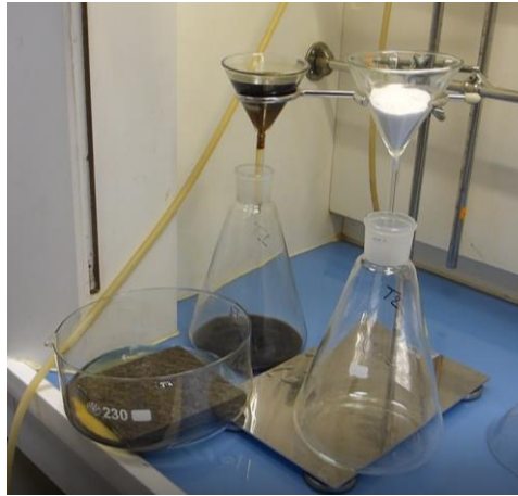
Figure 6 Oil extraction in dichloromethane and drying over sodium sulphate
