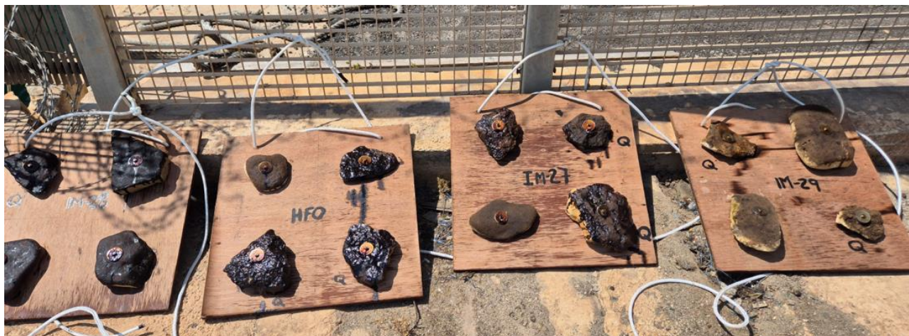
Figure 16 Wooden frames supporting the rocks recovered with the studied oils
