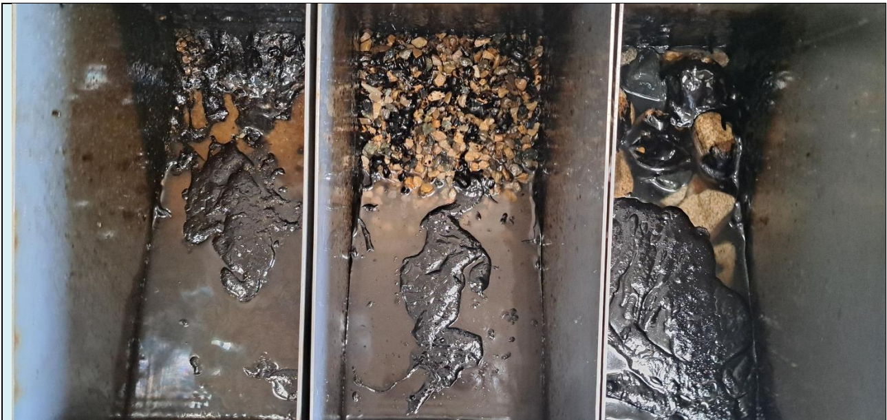
Slow remobilisation of the oil layer covering the sediment. The oil trapped in the sediment does not resurface. Manual agitation of the sediment allows an easy remobilisation of the trapped oil, leaving cleaned sediments.
