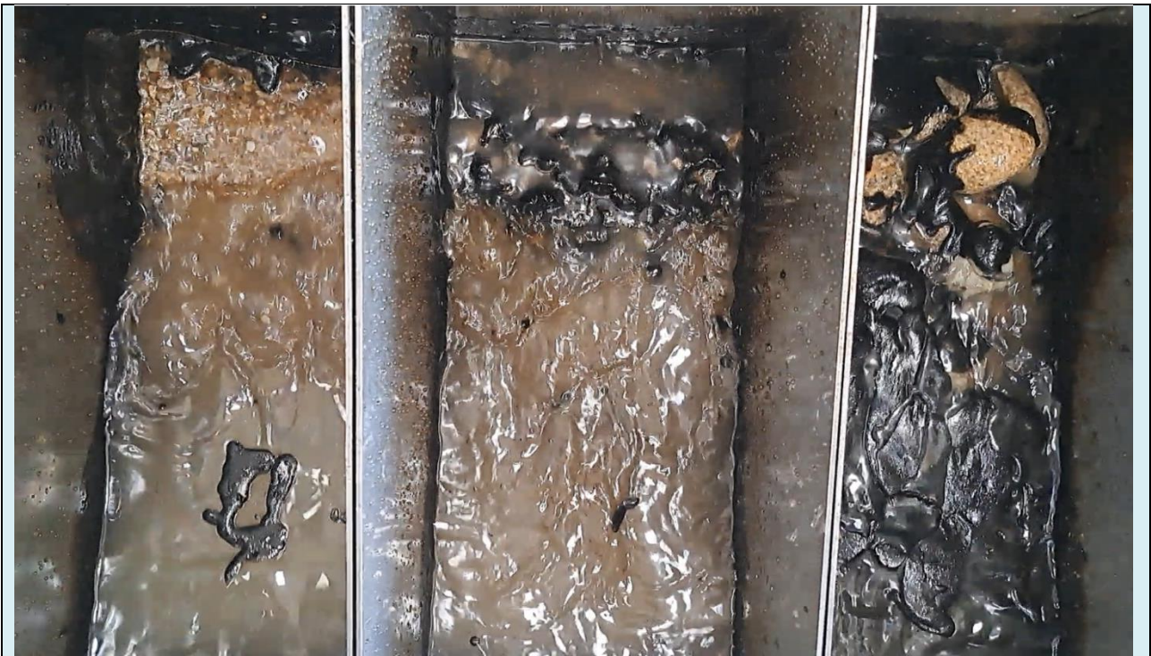
Slow remobilisation of the oil layer covering the sediment, leaving the surface of the sediment almost clean. Oil trapped in the sediment does not resurface. Manual agitation of the sediment allows an easy remobilisation of the trapped oil, leaving cleaned sediments.
