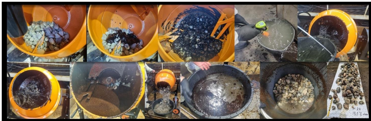
Figure 27: Small-scale test 4 - oiling and tumbling of pebbles in a concrete mixer.
