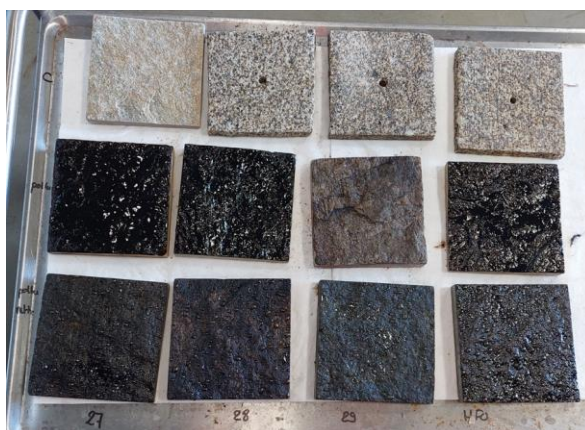
Figure 8 Pollution of the eight tiles used for ecotoxicology tests, after cleaning with the high-pressure washer of one of the two tiles per oil (bottom line) (note: the tile used with IM-29 that was not high-pressure washed shows a high degree of penetration)
