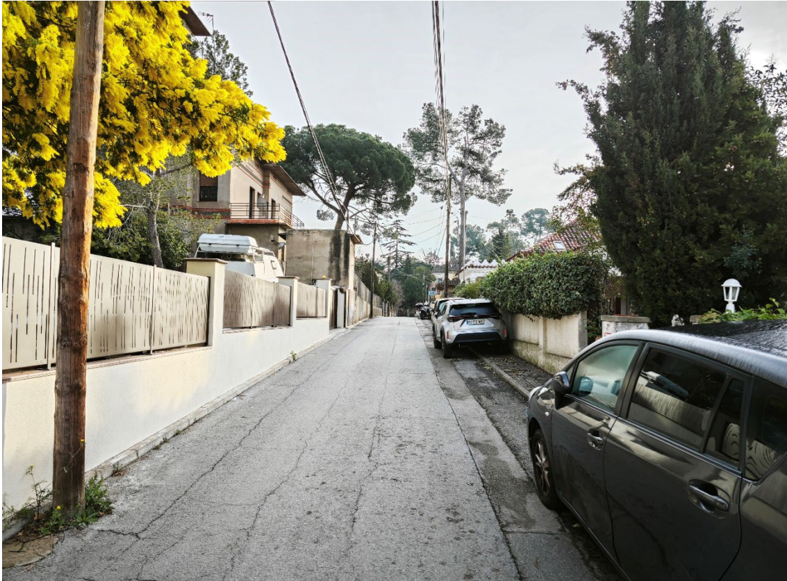
Figure 4. A street of la Floresta. The width of the streets is a critical factor, which makes it difficult to generate two-way circulation. The presence of parked vehicles further complicates the situation, as it reduces space and restricts movement, hindering both evacuation and the access of firefighting teams during an emergency.
