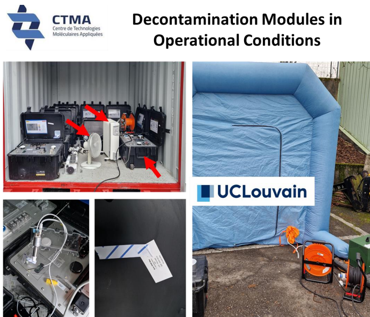
Figure 6. On-site decontamination was conducted inside a small container and a tent deployed at the Luxembourg Civil Protection Facility. Colorimetric indicators were placed at various locations to monitor VHP exposure. As indicated by the red arrows in the top-left panel, a small heater was placed beside the VHP spreading device to enhance ppm levels, while a fan ensured homogeneous hydrogen peroxide distribution within both structures
