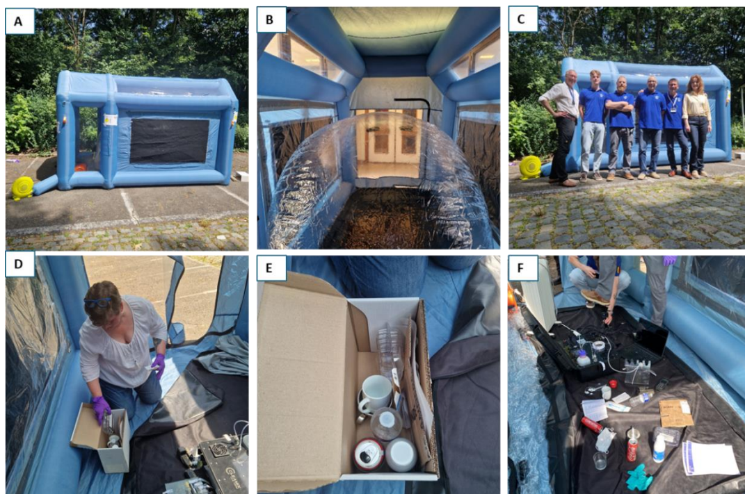
Figure 16. Double-confined inflatable setup for forensic testing.
