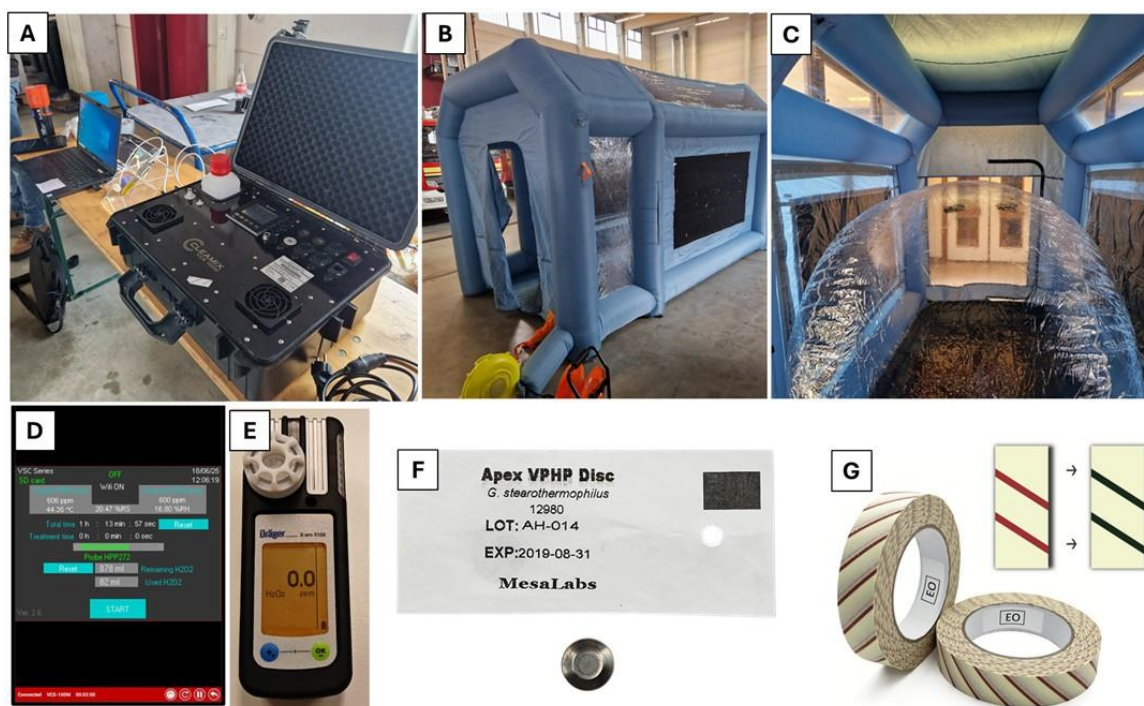
Figure 3. Main components of the on-site VHP decontamination system.
