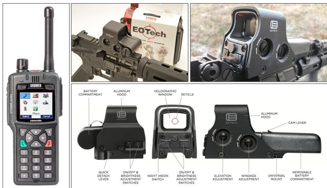
Figure 17. Electronics-sensitive police equipment tested for VHP decontamination.
